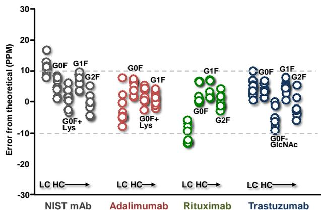
**Figure 1.** Scatter plot representing the PPM error from theoretical for each identified form for each therapeutic mAb. Each point represents one protein form. The points are colored and grouped on the X axis according to therapeutic. The data are jittered on the X axis for clarity.
