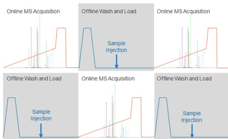
**Figure 1. Two-Column Switching Workflow using cHiPLC® system.** This easy-to-setup workflow provides up to a 2-fold increase in throughput. One column is used for running the biological sample, while the other column is regenerated offline.
