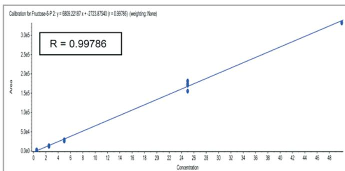
**Figure 8.** Calibration curve for Fructose-6-phosphate (200 nMolar - 200  $\mu$ Molar).
