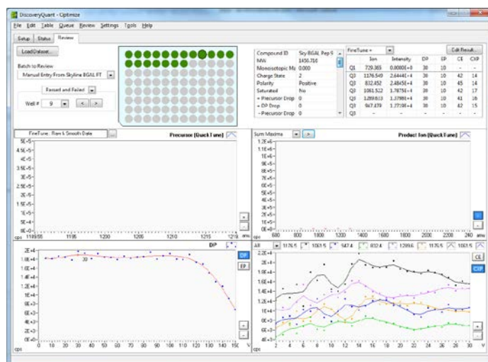
Figure 4. DP and CXP optimization data from the peptide APLDNDIGVSEATR using DiscoveryQuant™ FineTune.
