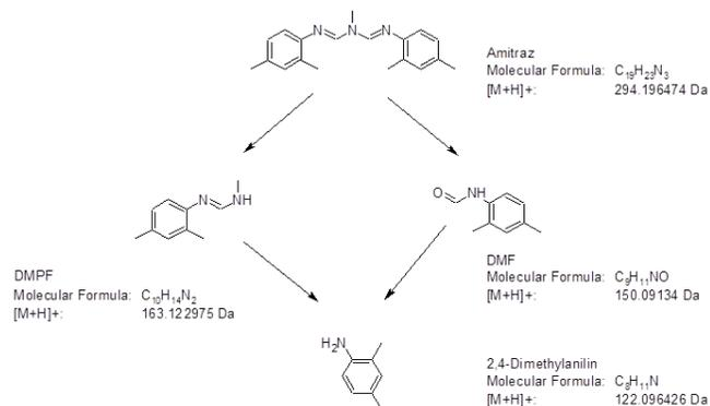
**Figure 5.** Chemical Structure of Amitraz and its metabolites
