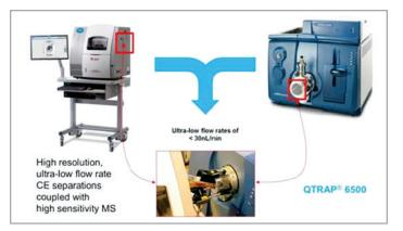
Figure 1. CESI-MS: CE integrated with the QTRAP<sup>®</sup> 6500 LC-MS/MS System
