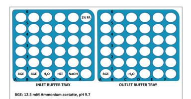
Figure 3. Scheme of the inlet and outlet buffer vial tray setup for the CESI separation.
