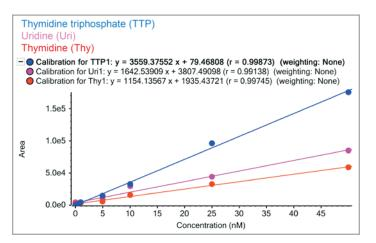
Figure 7. Calibration curves for the analyzed compounds. All analyte concentrations are ranging from 0 to 50 nM.
