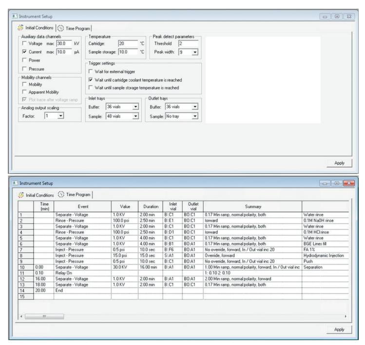
Figure 4. Separation method parameters. In step 10 and 12, use 2 psi of forward pressure. In steps 3, 5, 6 and 13 a low separation voltage is applied with 100 psi in both directions to rinse in parallel the capillary in the separation and conductive lines.
