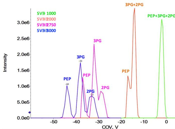
**Figure 2. Differential Mobility Spectrometry Resolves Isobaric Overlap.** The separation of 3-phosphoglycerate (3PG), 2-phosphoglycerate (2PG) and phosphoenolpyruvate using SelexION technology was tested using four different separation voltages (SV). Using isopropanol as a modifier reagent, high SV voltages were effective in resolving all metabolites.
