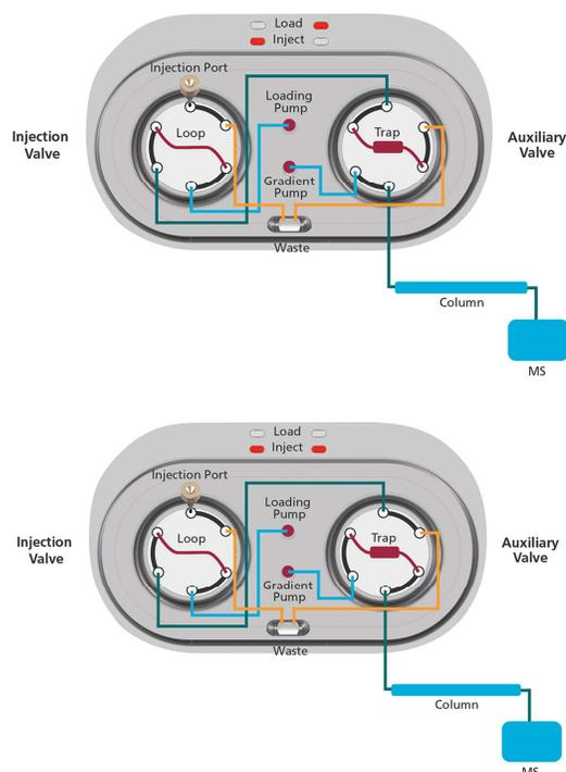
**Figure 1.** Valve positions for the trap loading part of the method (top) and the analysis part of the method (bottom).
