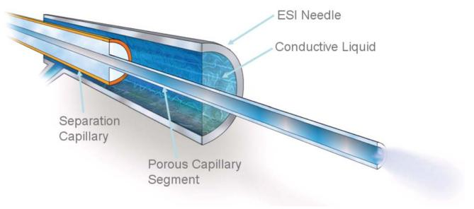
Figure 1. Schematic of the OptiMS capillary.
