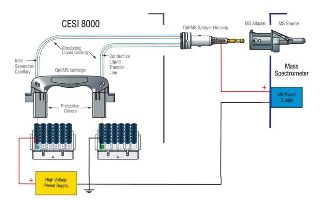
Figure 2: Schematic of the OptiMS Cartridge and retractable tip assembly. The data was generated on a prototype similar to the one shown above.
