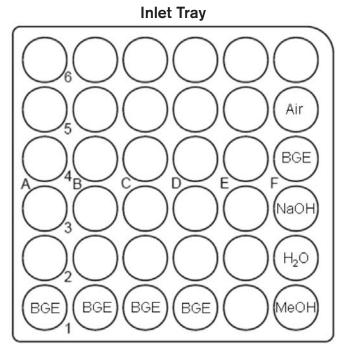
Figure 7: Buffer tray vial configuration for all methods.
