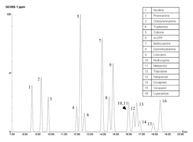
Figure 8: Total Ion Chromatogram (TIC) of the performance standard test mix.
