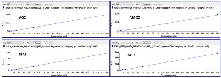
Figure 4: Matrix based calibration curve AOZ, AMOZ, SEM and AHD in Honey sample showing r = >0.99
