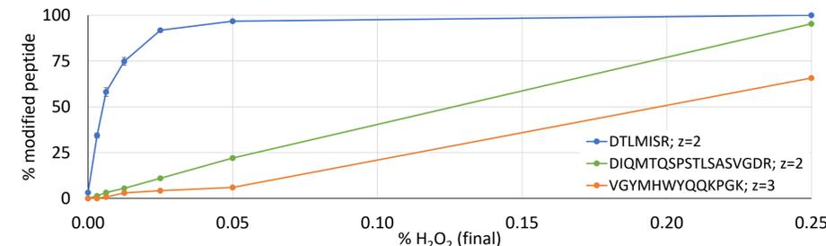
Figure 6. Mean percentages of different modified peptides based on XIC on MS level (n = 3). mAb samples were incubated with H<sub>2</sub>O<sub>2</sub> at 37° C for four hours prior to digestion.
