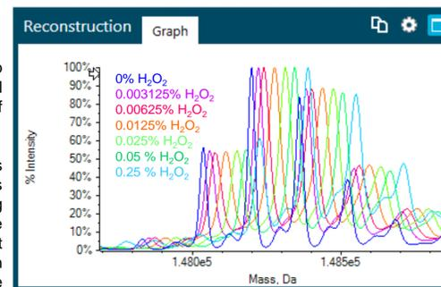
Figure 2. Reconstructed masses of intact mAb samples incubated with different concentrations of H<sub>2</sub>O<sub>2</sub> at 37° C for four hours.
