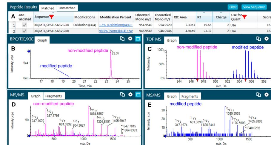
Figure 5. Evaluation of peptide DIQMTQSPSTLSASVGDR. mAb sample was incubated with 0.003125 % H<sub>2</sub>O<sub>2</sub> at 37° C for four hours prior to digestion. A: Table for automated calculation of percentage of modification B: Extracted ion chromatograms (XIC) on TOF MS level for modified and non-modified peptide. C: MS trace for modified and non-modified peptide. D: MS/MS data of non-modified peptide E: MS/MS data of modified peptide
