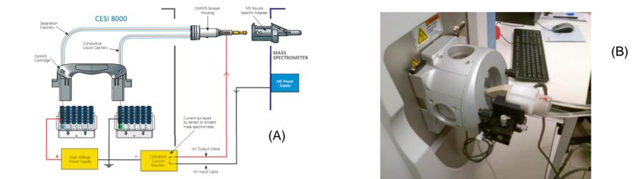
Fig. 1 A. Schematic representation of the CESI 8000 system. B. A Thermo Scientific™ nanospray source with an OptiMS sprayer adaptor
