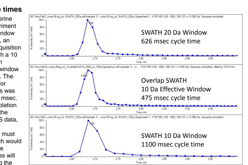
number of points across a peak). The demultiplexed MS/MS from overlap SWATH acquisition can approach the quality of a true 10 Da SWATH acquisition MS/MS, while having an improved cycle time.
