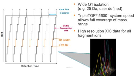
Figure 3. SWATH™ Scan Obtains MSMS data on all ions. By stepping the mass range in 25 Da increments, fragment ion chromatograms of all observed ions are collected.
