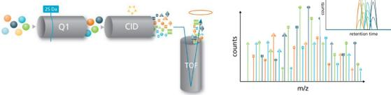
Figure 2. SWATH™ Scan Modality Overview. Standard MRM quant has 0.7 Da isolation on both quadrupoles. MRM<sup>HR</sup>, available on the 5600, still scans Q1 at a width of 0.7 Da but fragment ion chromatograms can be extracted from high resolution (>30K) MSMS scans at much narrower widths (0.007 Da) enabling higher selectivity. SWATH™ technology maximizes the use of MSMS resolution, extracting narrow fragment ion chromatograms from fragmentation of a wide isolation in Q1 (~25Da).
