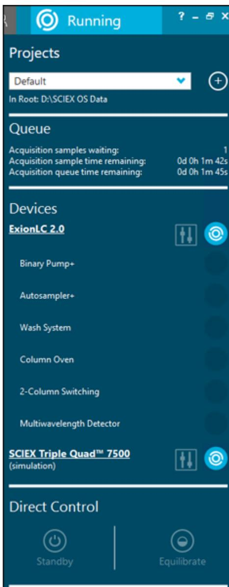
The Device Control dialog opens. It shows the real-time status of the devices in the ExionLC 2.0 system. Press **F1** for help.
