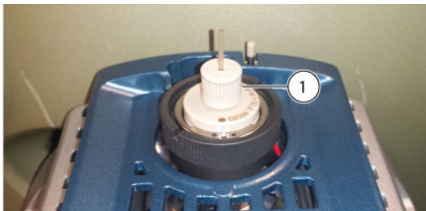
Figure 3-3 Bottom Fitting Installed
