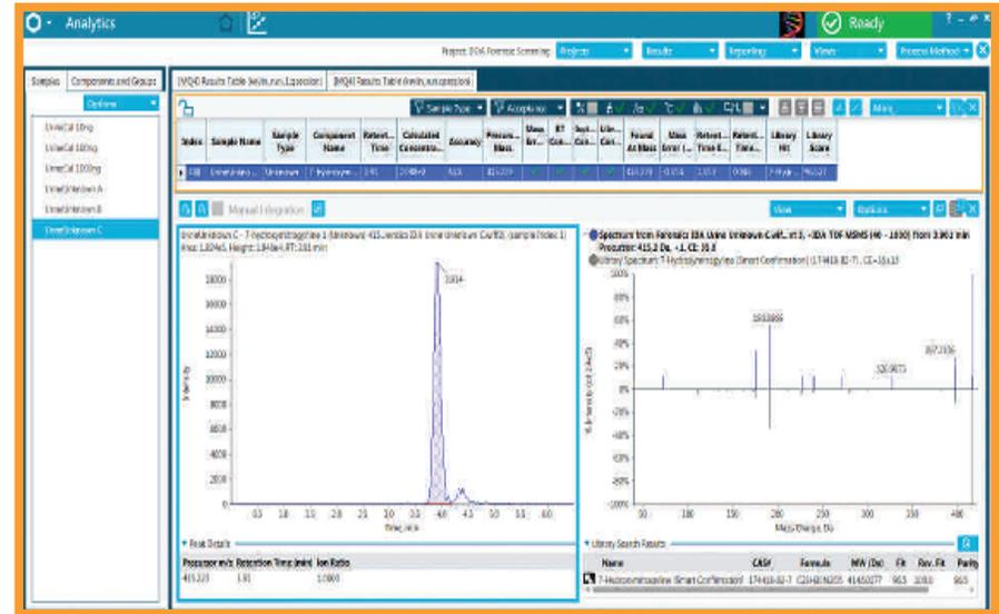
TOF MS and Information Dependent TOF MS/MS acquisition delivers reliable unknown identification of drugs in forensic samples.
