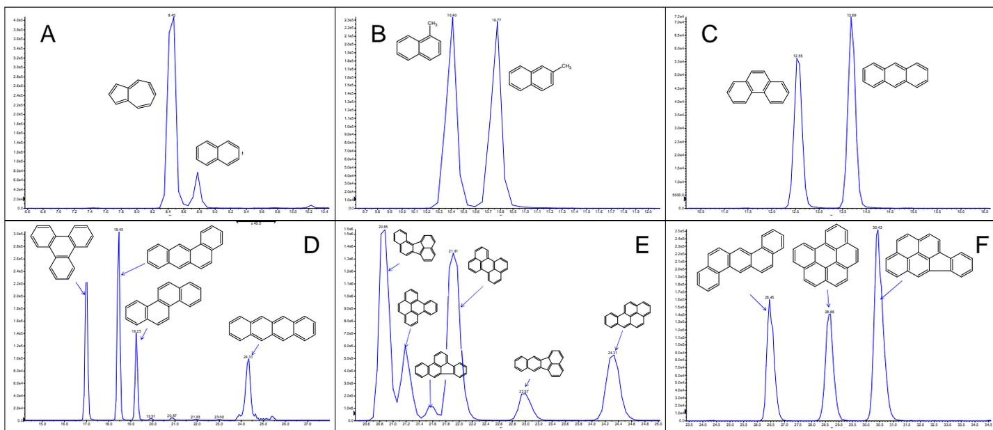
**Figure 3.** Separation of critical isomers using the developed LC method
