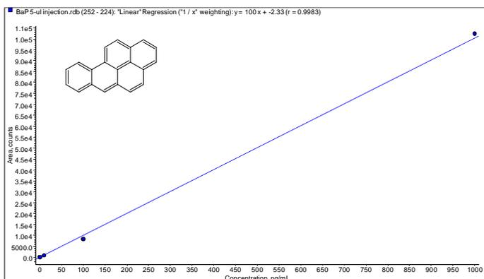
**Figure 4.** Calibration line of benzo(a)pyrene using triplicate injections into LC-MS/MS with APCI
