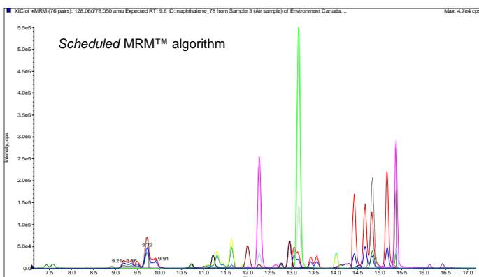
**Figure 6.** Detection of PAH, alkyl derivatives, and photo-oxidation products in an atmospheric particulate sample
